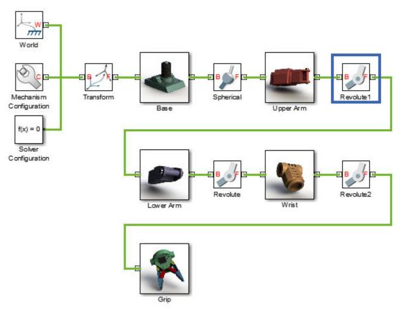
Joint blocks are assortments of joint primitives, basic yet complete joints of various kinds you cannot decompose any further—at least without losing behavior such as the
